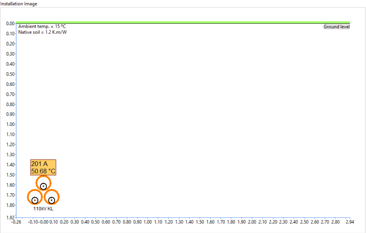
Figure 1 Buried installation arrangement (m)
